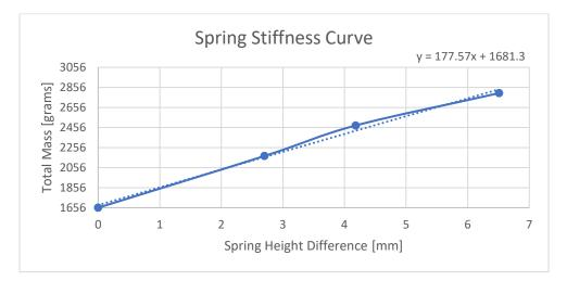
Figure 5. Spring stiffness curve
