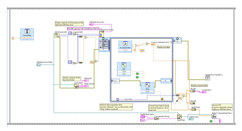
Figure 1. Block diagram z-axis acceleration data acquisition using NI MyRIO
