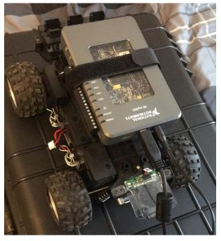
Figure 2. NI MyRIO with onboard accelerometer.
