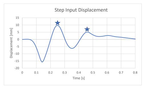
Figure 8. Step input response bouncing the vehicle
