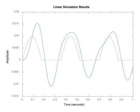
Figure 12. Simulated response, with the amplitude of displacement [m] as a function of time
