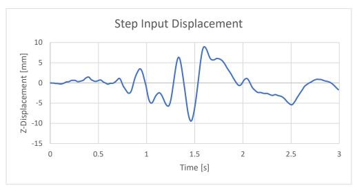
Figure 7. Step input response over a 1 cm bump at 0.47 m/s.
